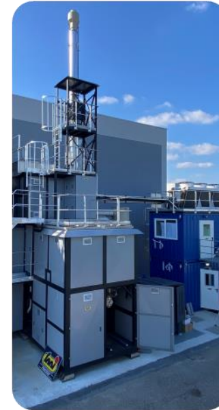
Heat exchangers Ash separation Flue gas treatment
